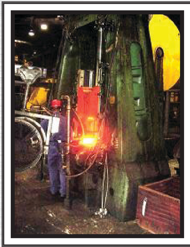
A #45 Power Forger in Operation
